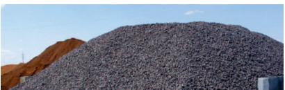
The 3/4" crushed stone is an aggregate size that has been crushed, reduced in size and screened through a 3/4" square screen. The material ranges in size from 3/4" to a #4 sieve, and a cubical product is needed for use in Superpave Mixes or projects that have a crush count specification.
