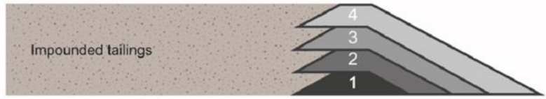
Centreline construction method
